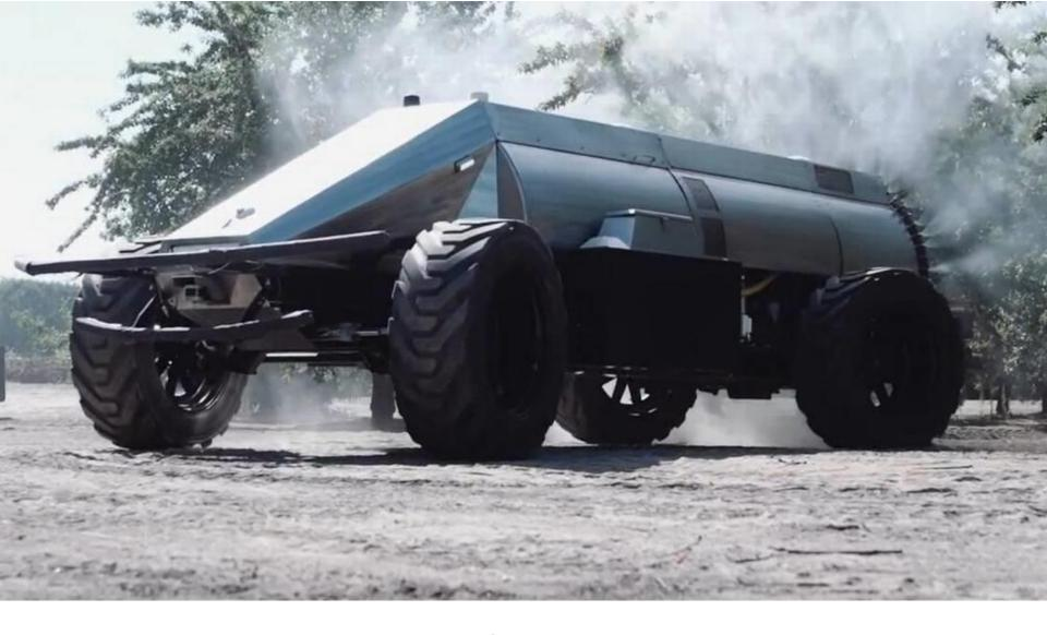
Robotic Airblast sprayer (Global Unmanned Spray System) from Crinklaw Farm Services, Kingsburg, CA
