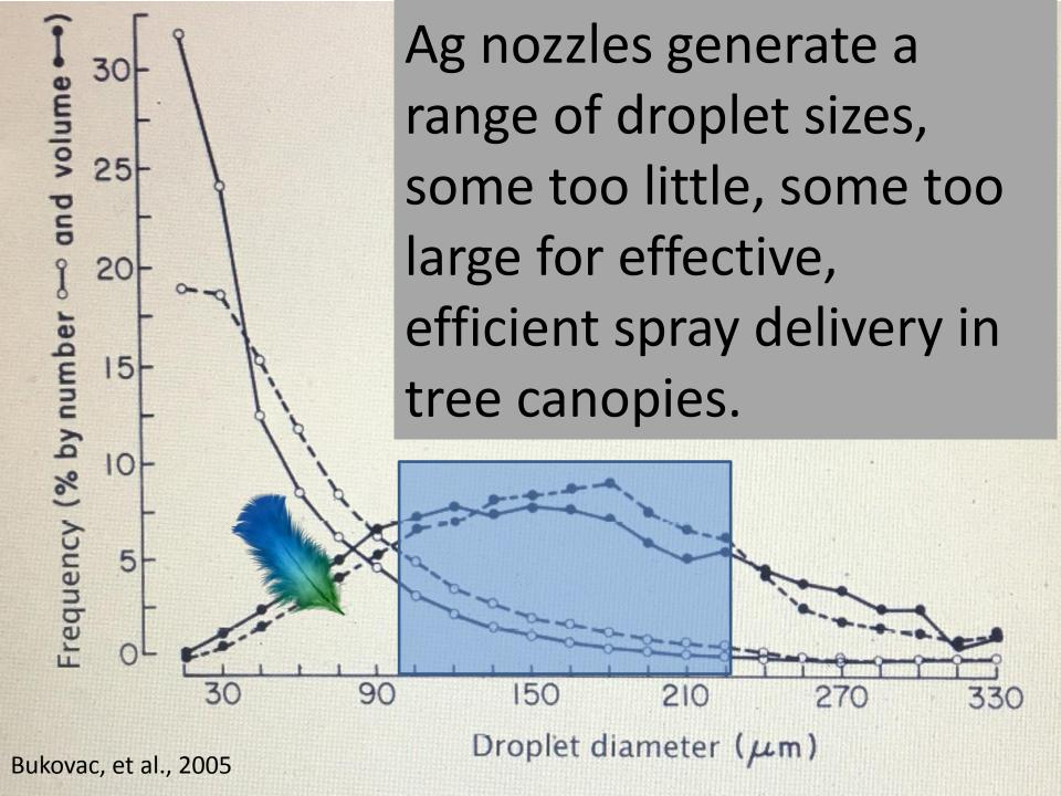
The smallest droplets tend to keep moving and not land (unless they are charged, move slow & get close to target).
